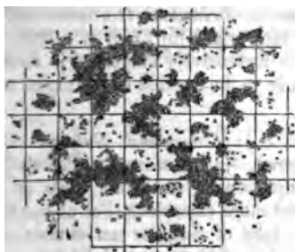
Microscopic appearance of pure precipitated sulphur. (The microneter squares are equal to those seen in Figs. 58 and 60.)
